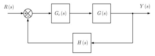
where the plant  $G(s) = \frac{G_o}{1 + \frac{s}{\omega_o}}$ , where  $G_o = 50$ ,  $\omega_o = 200$  rad/s and H(s) = 1. Transfer function  $G_c(s)$  represents the compensator.
