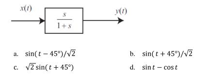
8. Referring to the figure below, the transfer function used for determining gain and phase margin from the Bode plot is:
