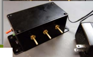
Analog circuit designed to create a sinusoidal air flow with variable amplitude and frequency.
